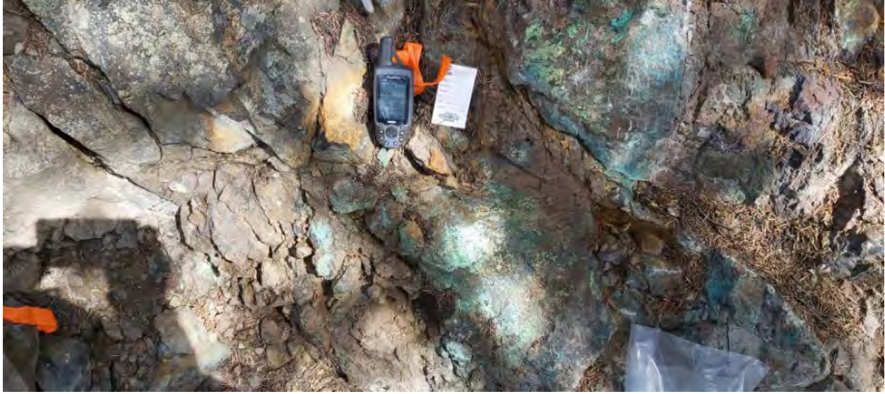
Figure 8. Sample #3249930 (Holmes Hill) - 1.2 m chip of magnetite-epidote skarn with lenses of fine grained chalcopyrite - occurs in old hand pits northeast of Mount Holmes
