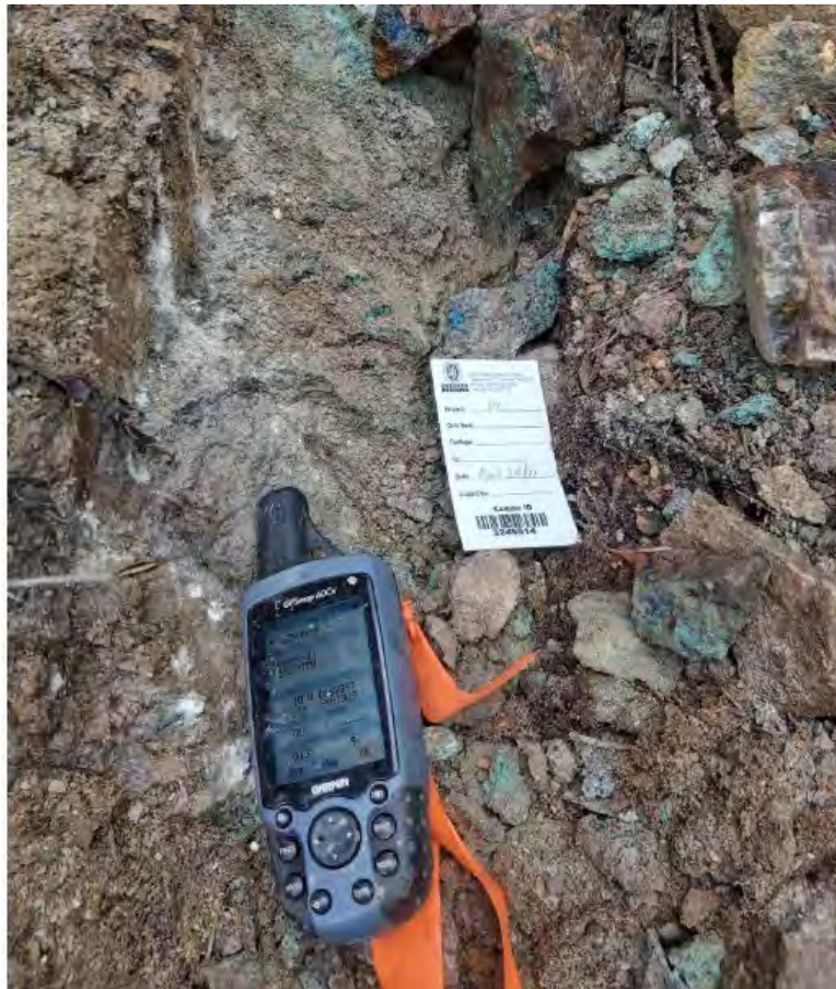
Figure 2. Sample #3249914 (Copper Farm). Chalcopyrite-malachite-azurite mineralization in a sheared granodiorite of the Bromley intrusion in contact with a felsic dyke.
