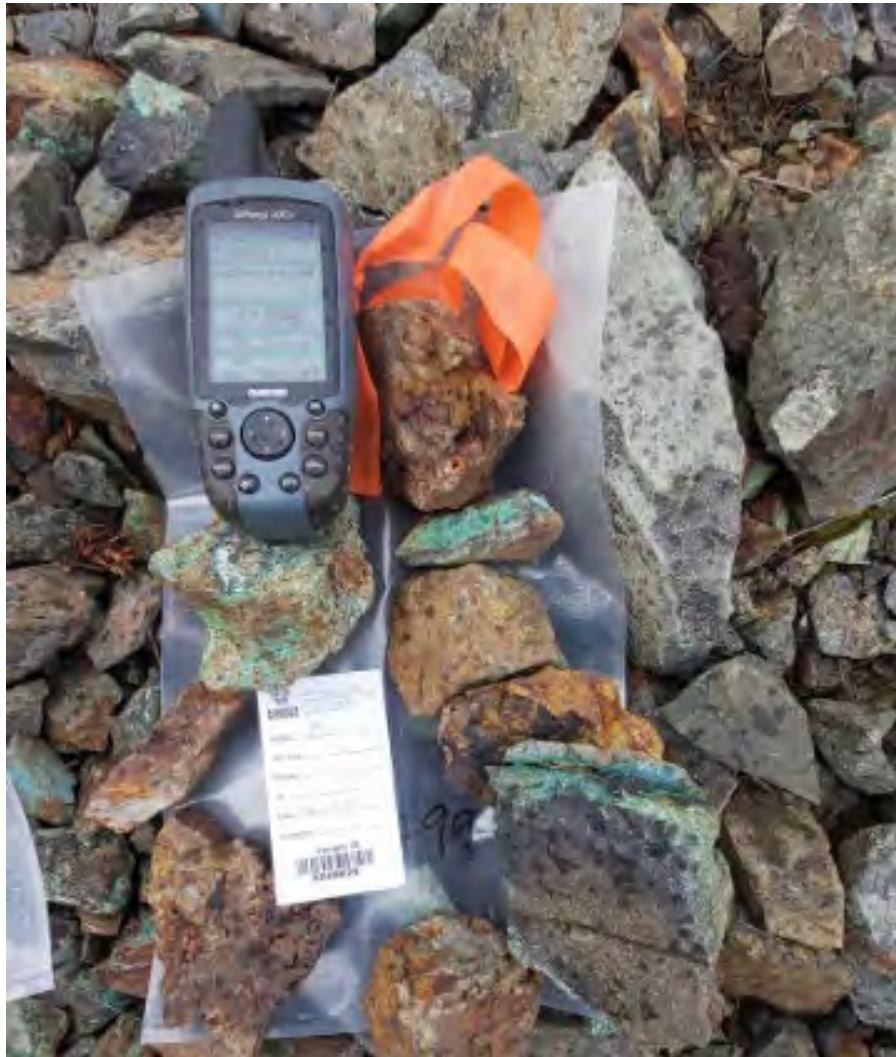
Figure 5. Sample #3249925 (Bud South): chalcopyrite-malachite-azurite mineralization in intermediate Nicola volcanics
