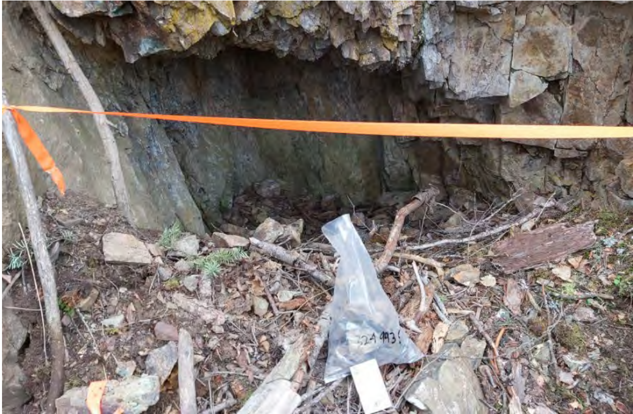
Figure 11. Sample #3249936 (Copper Farm) – a 1.2 m chip across sheared Nicola volcanics, black-limonite-quartz-carbonate veins, and 2-5 cm veins of chalcopyrite-malachite-azurite. This open cut pictured is directly beneath the sample.
