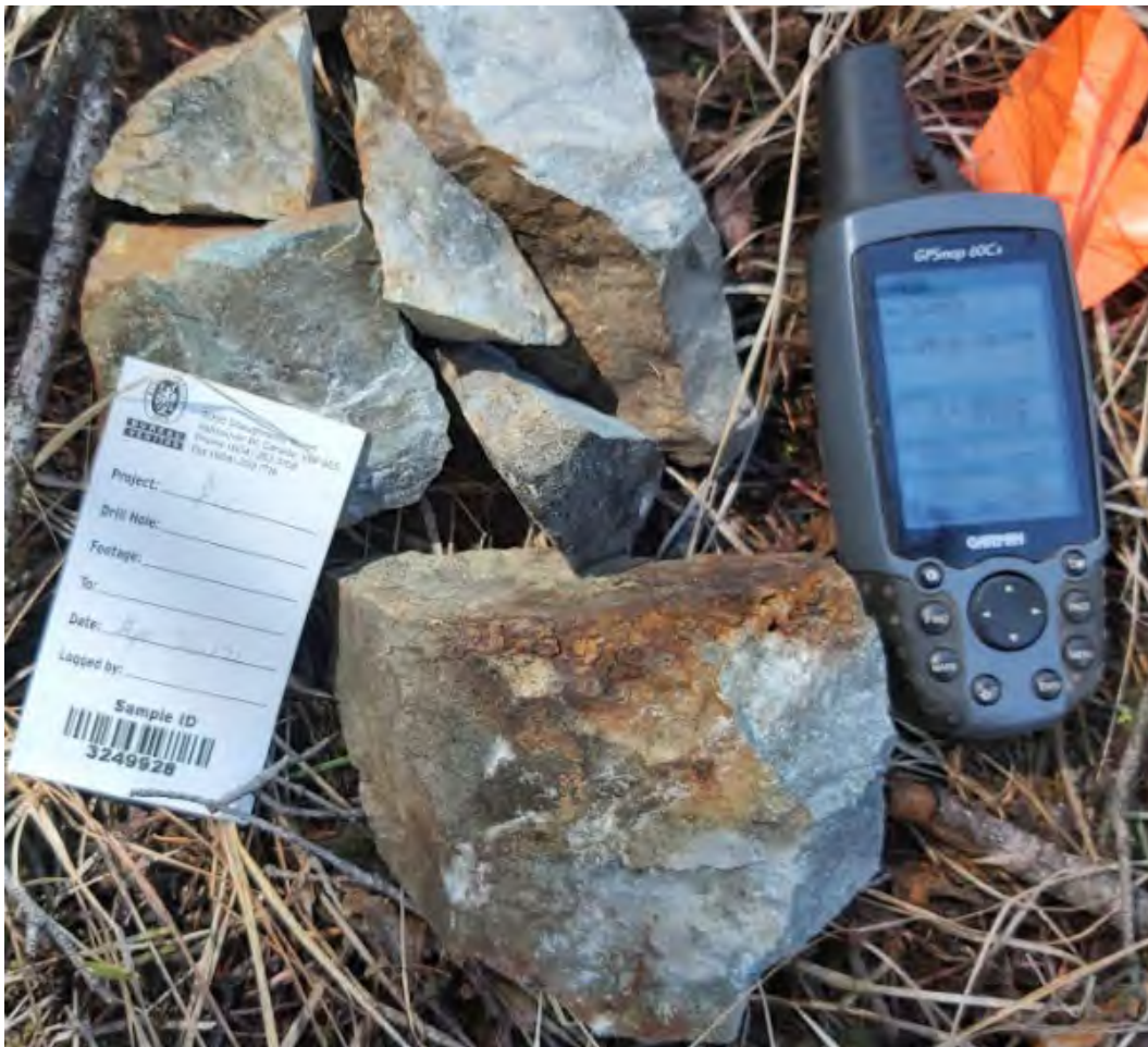
Figure 6. Sample #3249928 (Bonsai) taken from an old hand-pit. Cherty felsic tuffaceous rock with lenses of fine-grained pyrrhotite
