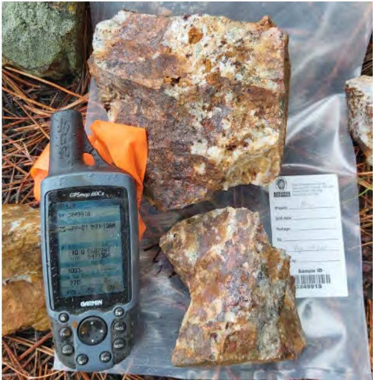
Figure 4. Sample #3249918 (Knob Hill) of chalcopyrite-galena mineralization in a quartz vein hosted by Nicola intermediate volcanics.
