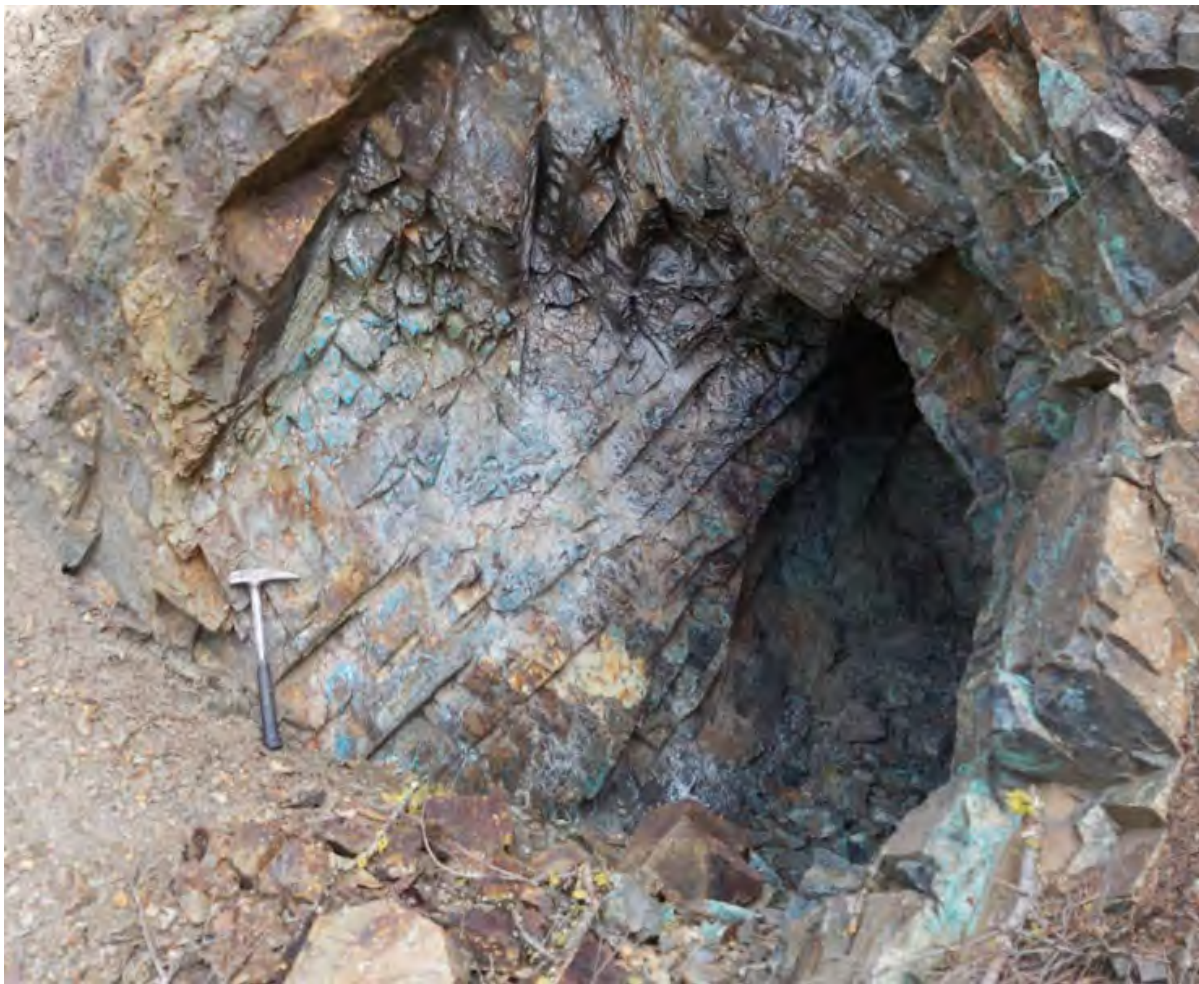
Figure 9. Small adit on Mount Holmes below Sample #3249932 - a grab of 10-20 cm wide quartz-carbonate vein with lenses of fine-grained chalcopyrite
