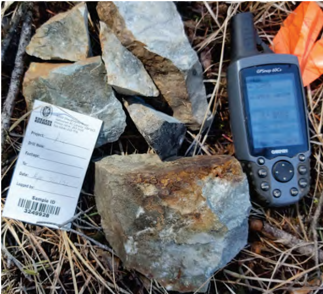
Figure 9-17. Rock sampling in old hand pits northeast of the Bonsai area, Sample 3249928 of cherty felsic tuffaceous rock with lenses of fine grained pyrrhotite.
