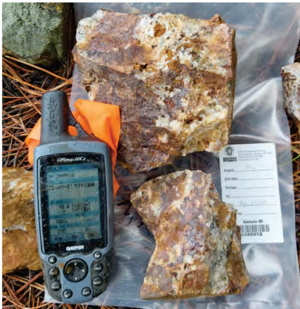
Figure 9-15. Sample 3249918 of chalcopyrite-galena mineralization in a quartz vein hosted by Nicola intermediate volcanic rock.
