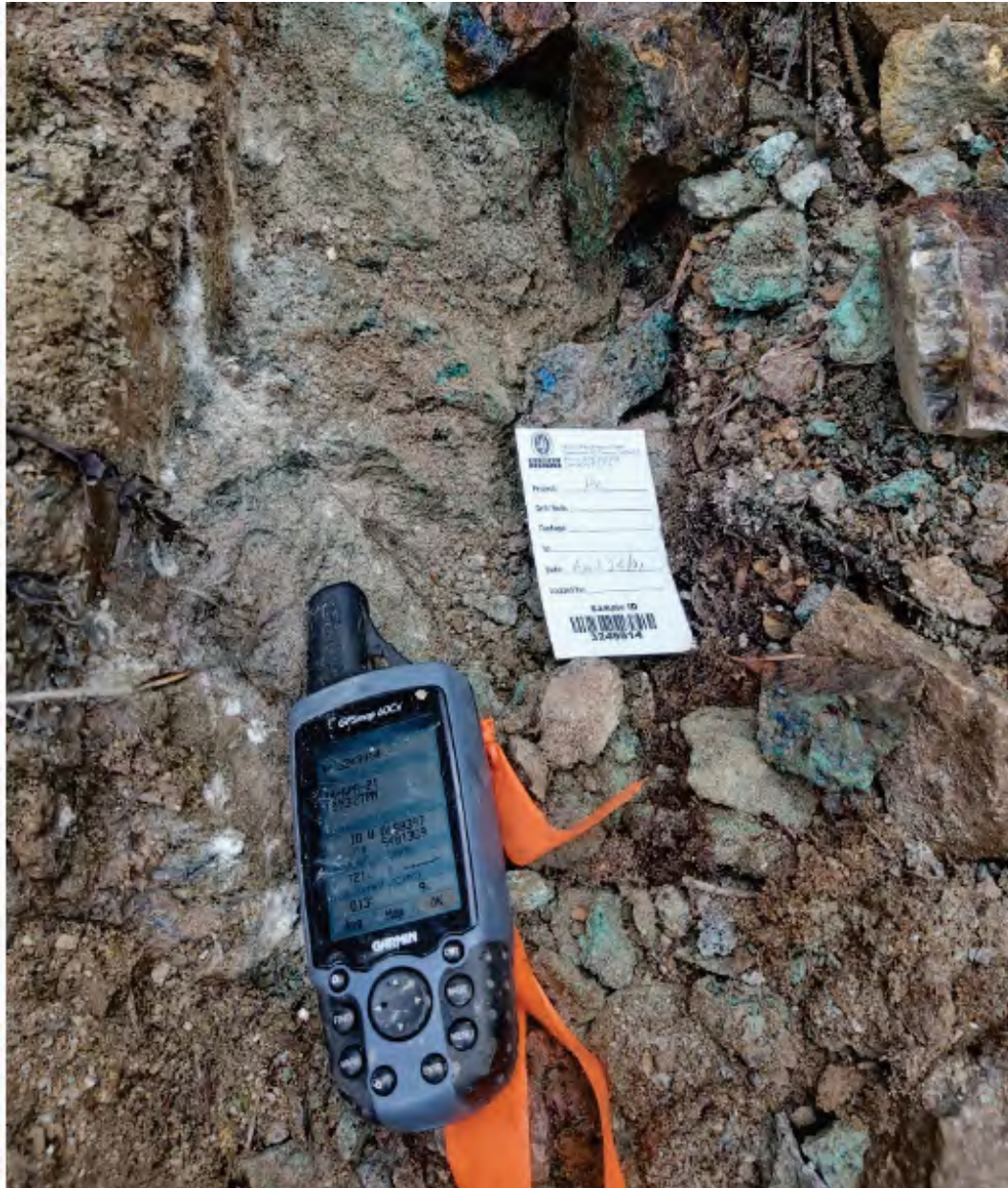
Figure 9-14. Sample 3249914 of chalcopyrite-malachite-azurite mineralization in a sheared granodiorite of the Bromley intrusion in contact with a felsic dyke.
